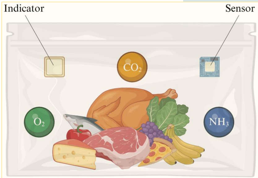
Figure 3.8 Gas Sensor and Indicator in Food Packaging, adapted from Wonyoung H. 2024
