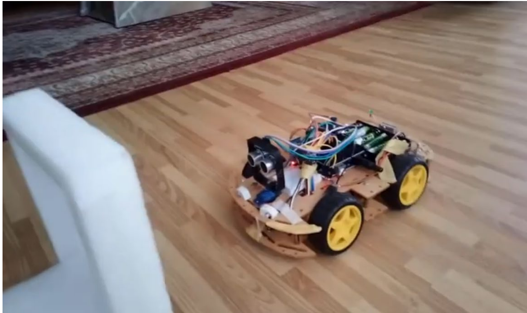
Figure 2.3.1: Robot with Sonar Obstacle Detection and Follow-Me
