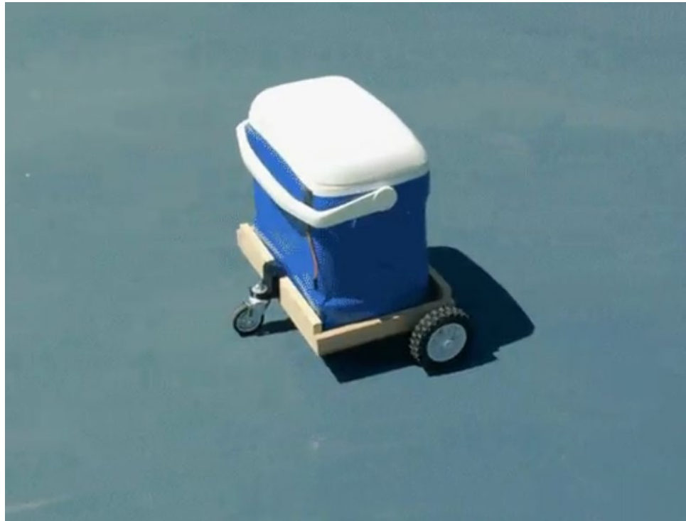
Figure 2.3.2 : Autonomous "Follow Me" Cooler
