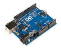
Arduino UNO is a microcontroller board based on the ATmega328P. It has 14 digital input/output pins (of which 6 can be used as PWM outputs), 6 analog inputs, a 16 MHz ceramic resonator, a USB connection, a power jack, an ICSP header and a reset button. It contains everything needed to support the microcontroller; simply connect it to a computer with a USB cable or power it with a AC-to-DC adapter or battery to get started.
