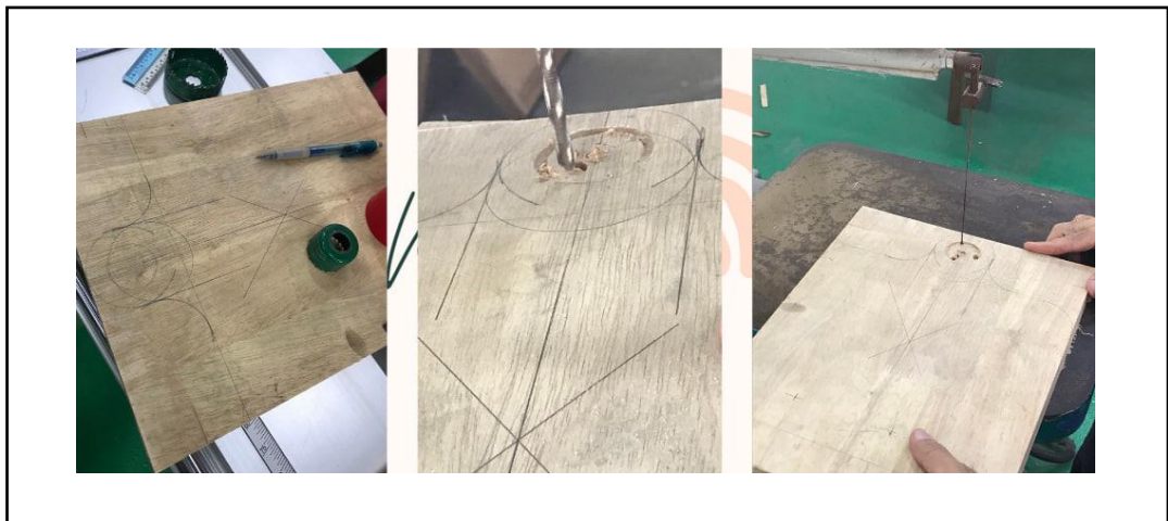
Figure 15 :Cut hole parts for handles with scroll saw machine
