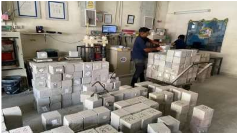
3.2.1.1 Concrete Compressive Strength
