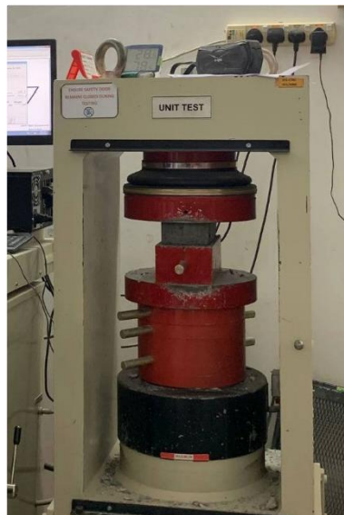
Figure 3.6: Digital compressive machine is used to measure the value of the compressive strength of brick
