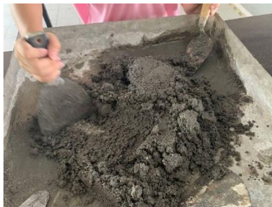
Figure 3.3: Cement, sand, crushed waste glass and water are mixed together
