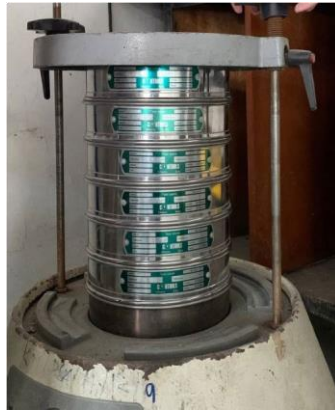
Figure 3.5: Sieving process to segregate the crushed waste glass
