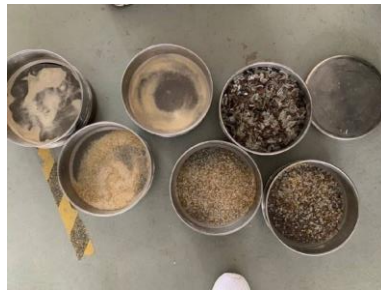
Figure 3.2: The glass particles are separated to a certain size after the sieving process
