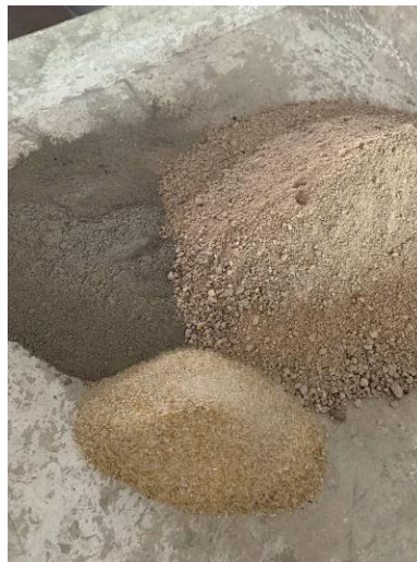
Figure 3.3: the materials of cement, sand, and 15% of crushed waste glass
