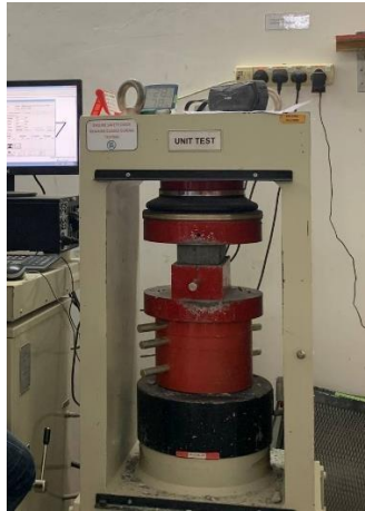
Figure 3.5: The compressive test by using the machine
