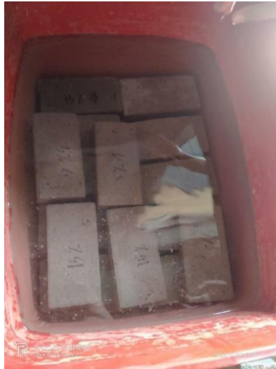
Figure 3.6: the place to put the sand brick in water absorption test
