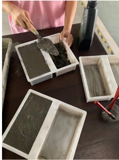
Figure 3.4: Process of putting the mixture into the mold
