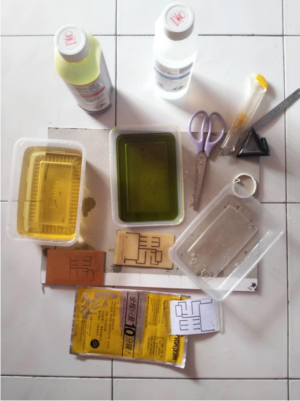
Figure 3.15: Etching of PCB
