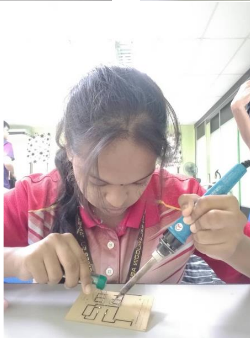
Figure 3.17: Soldering of PCB
