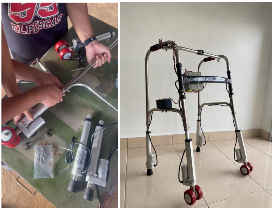
Figure 3.3.11 – Connection of Walking Frame Parts
