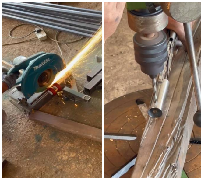
Figure 3.3.10 – Cutting Parts of the Walking Frame
