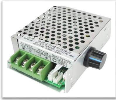
FIGURE 3.4.4: DC Motor Controller
