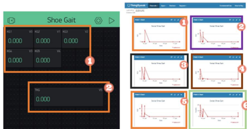
Figure 4: Interface of IoT implementation using Blynk and Thingspeak application for detecting the pressure of resistive pressure sensor
