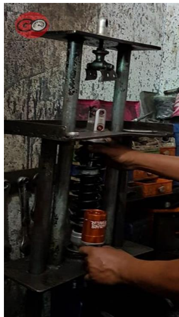
Figure 2.3 Semi Manual Absorber Remover
