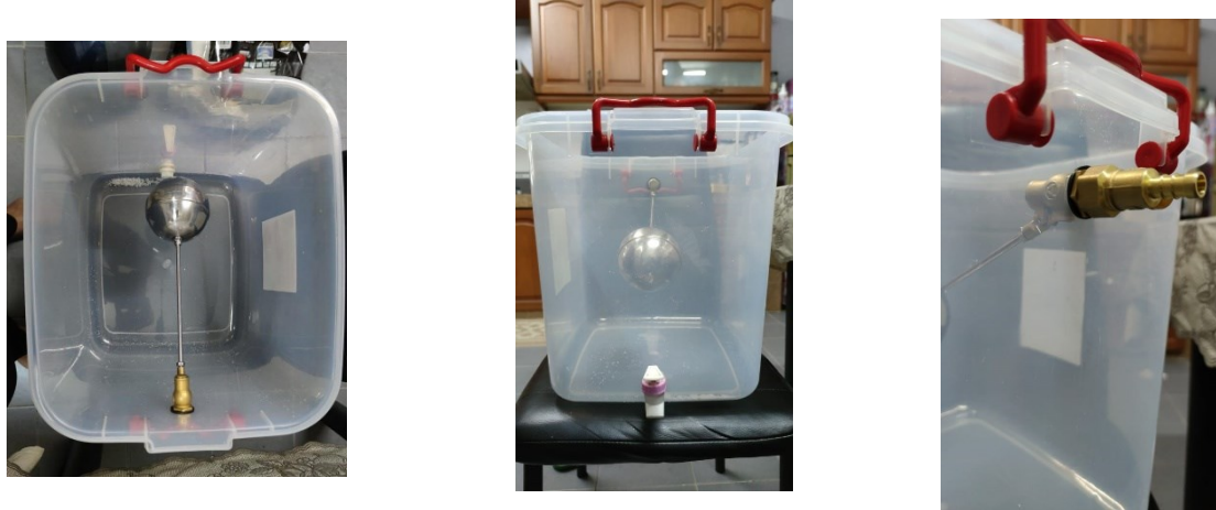
Figure 3.4 i. Manufacture of tank to collect water
