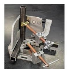
Welding clamps are holders of metal sheets or legs that tie two parts of materials securely together temporarily. In a close alignment, the clamps help you to solder parts together. They are particularly useful for dealing with large sheets and metal frames that are hard to keep together by hand alone. But that doesn't mean that they're useful just for bigger shields.
