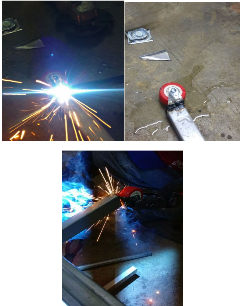
Figure 3.3 ( Installation of Wheels by using MIG welding)
