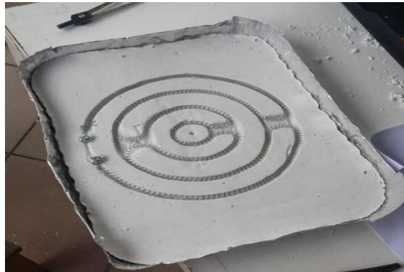
Figure 2.4.2 – Base of heat element
