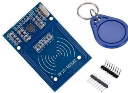
Figure 3.3 RFID RC522 Module with a RFID tag
