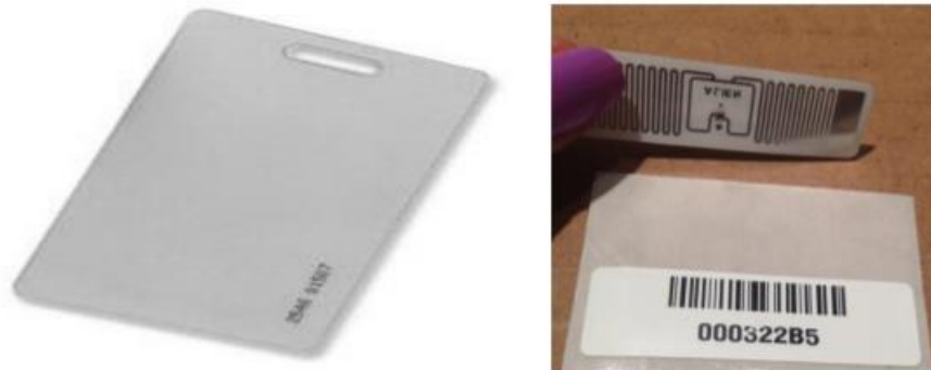
Figure 3.8 RFID Passive Tag
