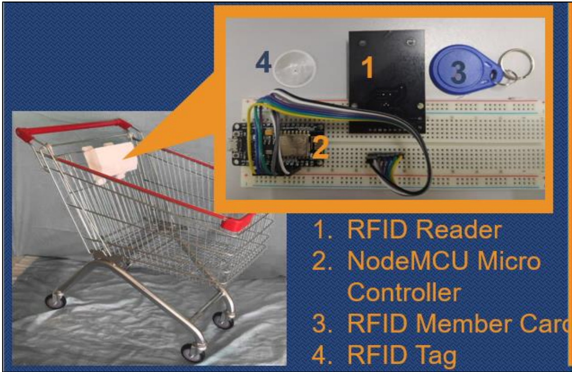
RFID Grocery Cart's RFID Device main Components.
