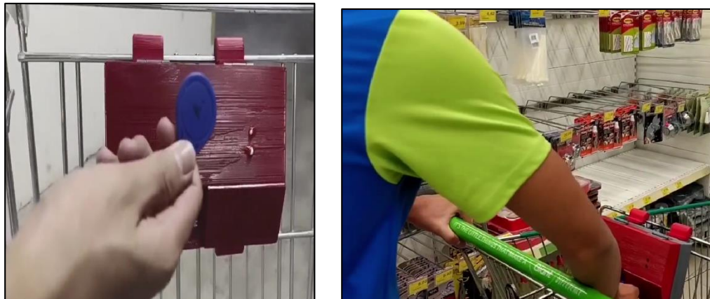
Figure 4.1 customer scanning RFID tag through RFID Scanner.
