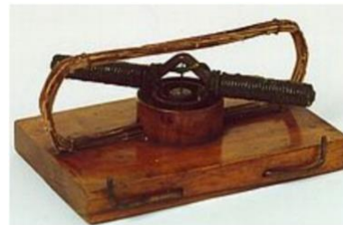
Jedlik's "lightning-magnetic self-rotor", 1827 (the world's first electric motor)
