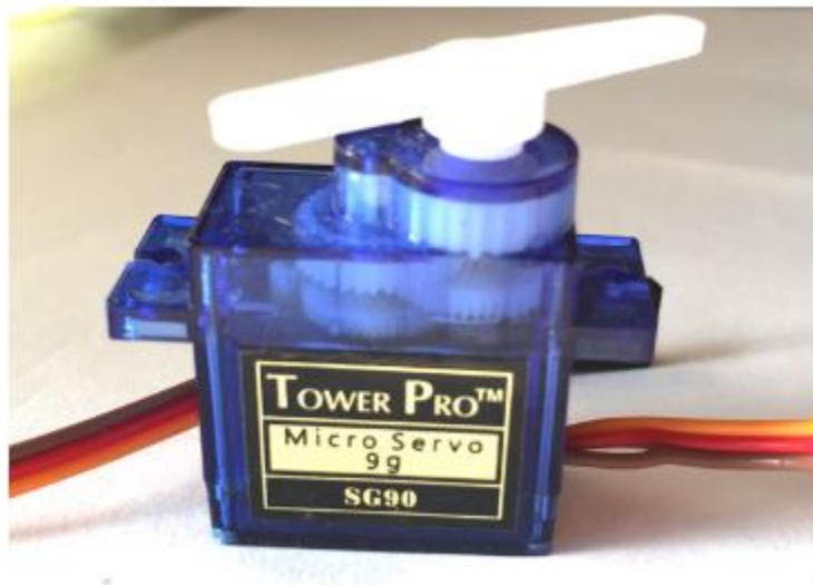
Figure 3.13 Tower Pro SG90 Micro Gear Servo
