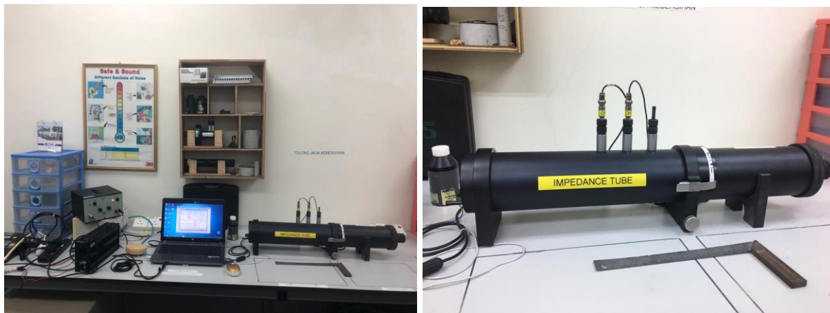
Rajah 3.2 Alat Impedance Tube
