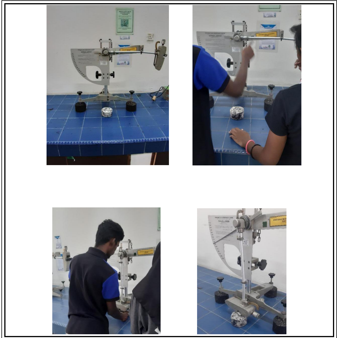
Figure 3.4.3.2: Skid resistance test
