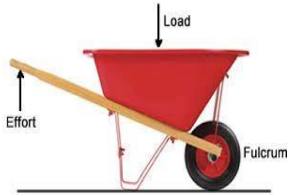
Figure 7.0: Concept of lever in a wheelbarrow
