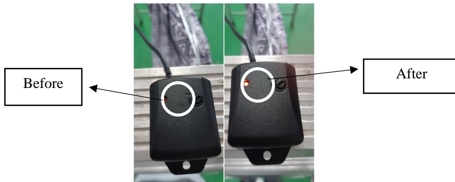
Figure 3.22: Before and after the vibration sensor detects any movement in the cradle
