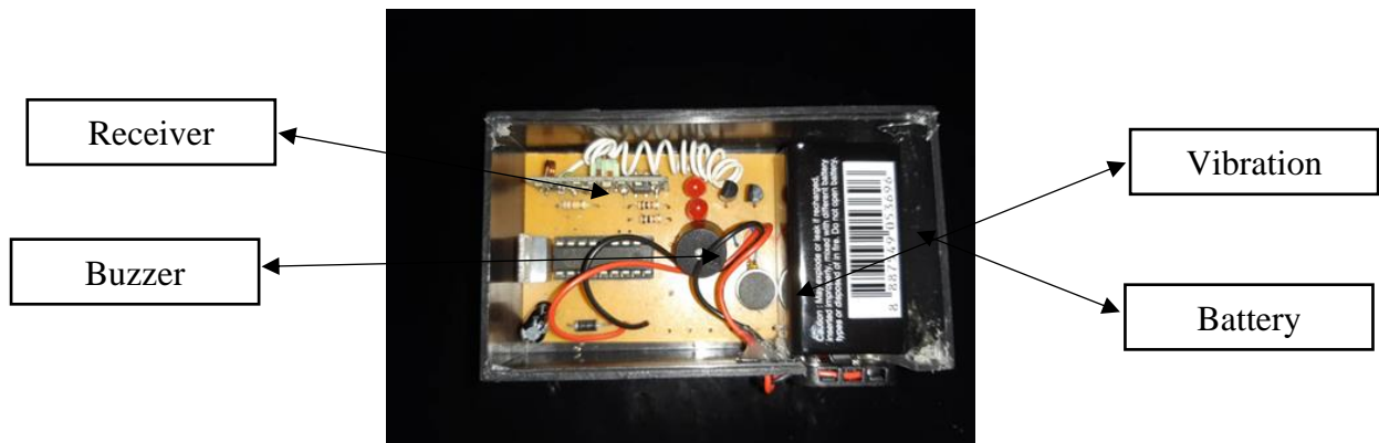
Figure 3.5: Components inside the remote alarm
