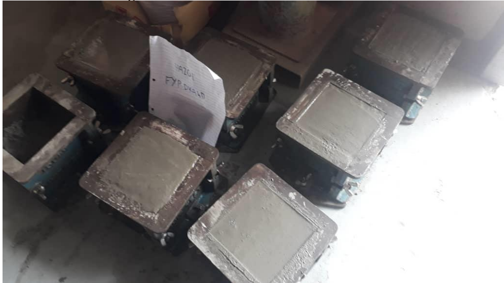
Figure 3-12: Concrete Cube in Mould
