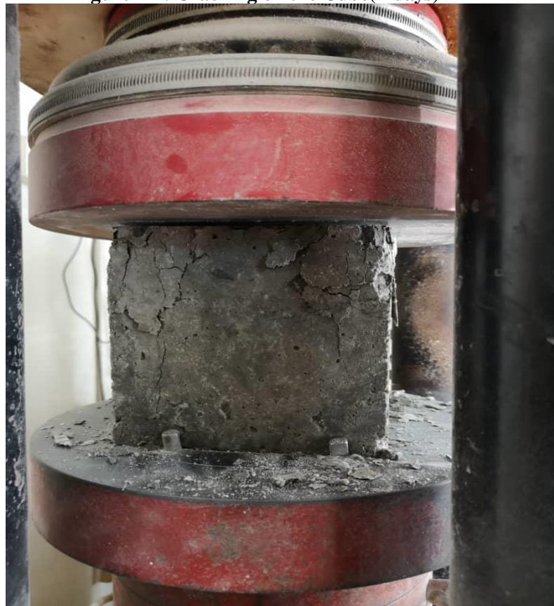
Figure 4-1: Cracking on the Cube(7-days)
