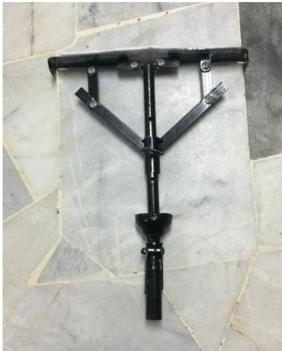
Figure 1.4 PAP for painting between wall and ceiling
