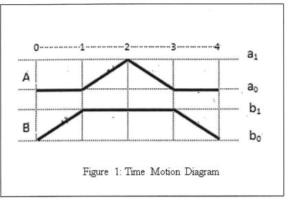
(a) Based on **FIGURE 1** of time motion diagram above, draw the sequence movement.
